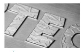
These plates are specially created to allow our customers to introduce personalised textures and marks on the self-adhesive materials and cardboards. The plates are placed in the magnetic cylinders and perform a debossing process on the material surface with the texture applied on the metal plate. The different possibilities for personalisation are almost endless, allowing narrow details, down to 0.1mm marks on the material surface.
